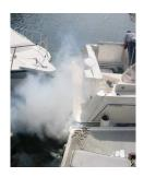
White smoke – is a fog of very small fuel droplets due to poor quality fuel, injector/valve timing problem, burnt valves, or bad gaskets allowing coolant into the cylinders
